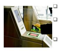
Display for guiding pax to swipe boarding passes on the scanner Scanner is capable of reading 2D, AZTEC barcodes to support paper printed and mobile boarding passes Flaps open and close to let pax board or to stop boarding the plane
